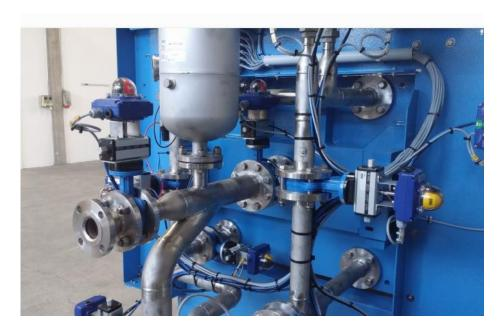
Cake blowing (or cake drying) is an optional which involves the insertion of compressed air (at 6/8 bar) inside the panels, after the filtration phase.
